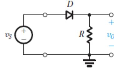
[8] A symmetrical square wave of 3-V peak-to-peak amplitude and zero average is applied to a circuit resembling that in Fig. 1 and employing a 100- $\Omega$  resistor. What is the peak output voltage that results? What is the average output voltage that results? What is the peak diode current? What is the average diode current? What is the maximum reverse voltage across the diode?
